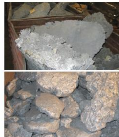
The reclamation system turns waste (top) into reusable metal (bottom).
